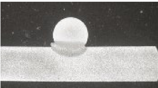
Fig. 3 - Cross section of the weld between a longitudinal wire and a ring..
