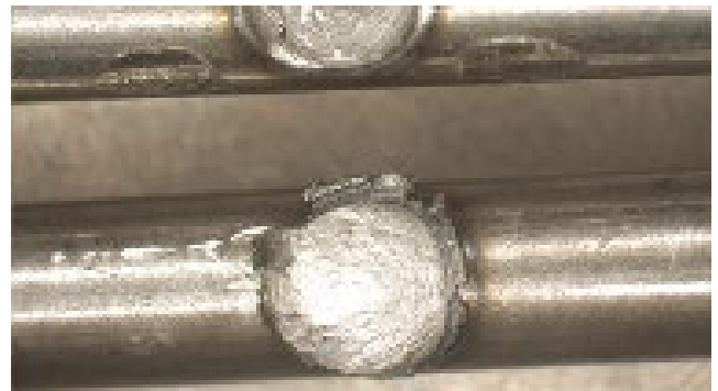
Fig. 2 - Tensile test of a joint made between a longitudinal wire and a ring.
